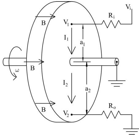
Fig. 2. Simplest form for the dc transformer is composed of a single spinning disk in a magnetic field with two sliding contacts on the disk face.
