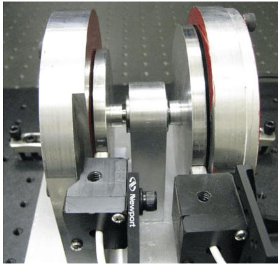
Fig. 3. Small scale device was constructed to demonstrate the dc–dc transformer concept using a pair of conducting disks spinning in a magnetic field.
