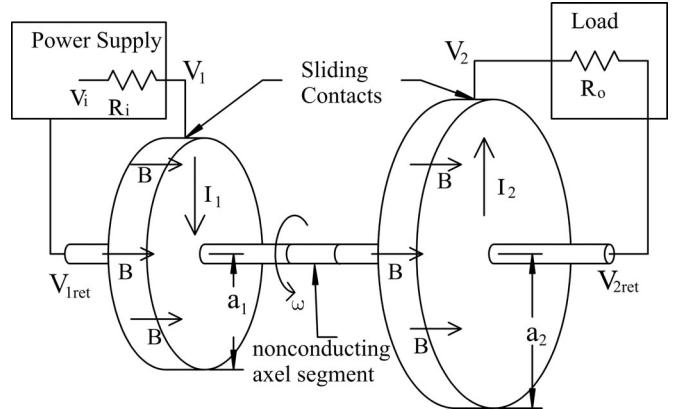
Fig. 1. Simplest isolated form of the dc transformer consists of two mechanically connected spinning disks located in a uniform magnetic field.
